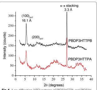
$\begin{tabular}{ll} \textbf{Fig. 6} & X-ray & diffraction (XRD) patterns of PBDP3HTTPA and PBDP3HTTPB powders \\ \end{tabular}$
