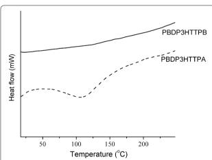
**Fig. 5** Second-heating run DSC curves (exo up) of PBDP3HTTPA and PBDP3HTTPB DSC was performed under nitrogen atmosphere at a heating rate of  $10 \, ^{\circ}\text{C}$  min $^{-1}$
