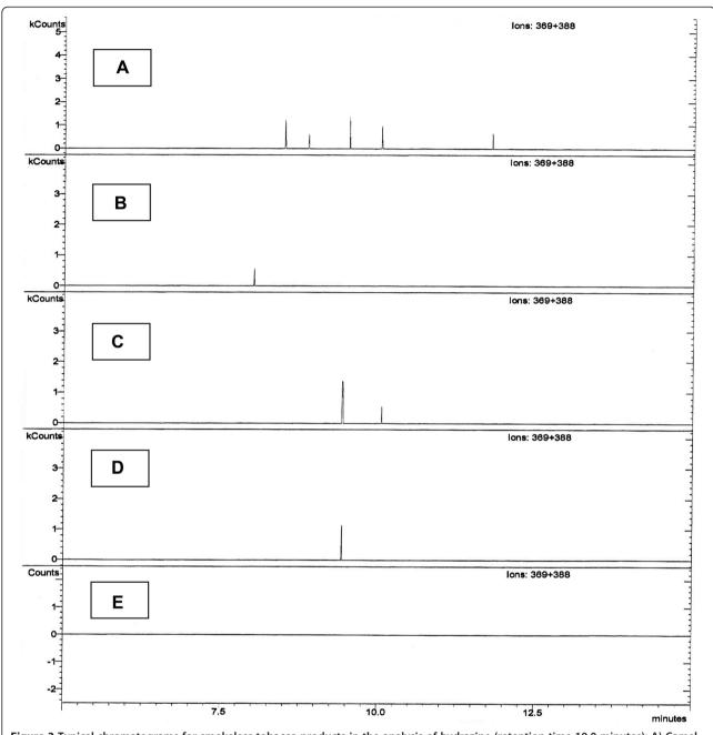
Figure 3 Typical chromatograms for smokeless tobacco products in the analysis of hydrazine (retention time 10.0 minutes); A) Camel Frost Snuff, B) Camel Mellow Snuff C) Marlboro Mild Snuff, D) Marlboro Peppermint Snuff, E) Marlboro Rich Snuff.
