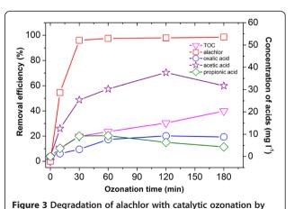
Cu/Al<sub>2</sub>O<sub>3</sub> powder and the corresponding acids produced: ( $\square$ ) alachlor; ( $\nabla$ ) TOC; ( $\stackrel{\leftarrow}{\nabla}$ ) acetic acid; (o) oxalic acid; ( $\diamond$ )propionic acid. T: 20°C, Alachlor concentration: 100 mg L<sup>-1</sup>, the dosage of Cu/Al<sub>2</sub>O<sub>3</sub> powder: 0.27g L<sup>-1</sup>.
