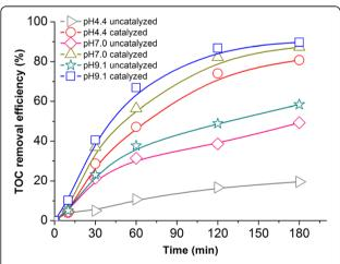
Figure 6 Influence of pH on TOC removal during catalyzed and uncatalyzed alachlor ozonation: ( $\triangleright$ ) pH 4.4 uncatalyzed; ( $\bigcirc$ ) pH 4.4 catalyzed; ( $\bigcirc$ ) pH 7.0 uncatalyzed; ( $\bigcirc$ ) pH 7.0 catalyzed; ( $\bigcirc$ ) pH 9.1 uncatalyzed; ( $\bigcirc$ ) pH 9.1 catalyzed. T: 20°C, Alachlor concentration: 100 mg L<sup>-1</sup>.
