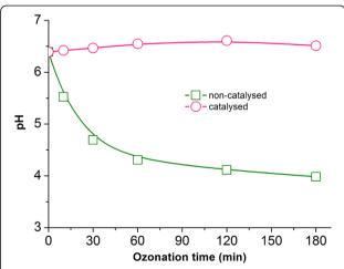
Figure 5 The shift in pH as a function of time before and after ozonation: (□) uncatalyzed process; (o) catalyzed process.
