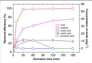
Figure 4 Degradation of alachlor with catalytic ozonation by  $Cu/Al_2O_3$ -honeycomb and the corresponding acids produced: ( $\Box$ ) alachlor; ( $\nabla$ ) TOC; ( $\not\simeq$ ) acetic acid; ( $\odot$ ) oxalic acid; ( $\diamond$ ) propionic acid. T:20°C, Alachlor concentration: 100 mg L<sup>-1</sup>.
