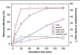
Figure 2 Degradation of alachlor when ozone was applied alone and acids produced in the reaction process: (□) alachlor; (▽) TOC; (☆) acetic acid; (o) oxalic acid; (⋄) propionic acid.
