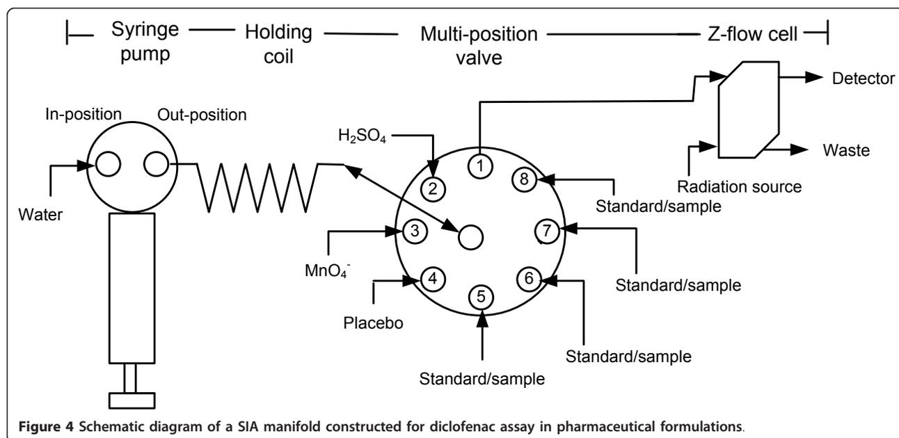
**Figure 4** Schematic diagram of a SIA manifold constructed for diclofenac assay in pharmaceutical formulations.
