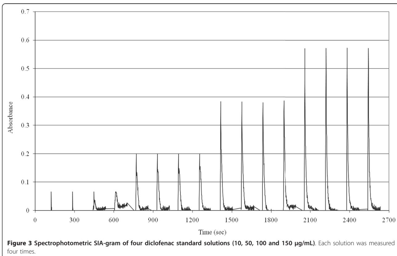
solutions (10, 50, 100 and 150 µg/mL) of diclofenac; each standard solution was measured four times.
